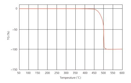
\*Thermal Gravimetric Measurement in dry air Raising Rate 10°C./min
