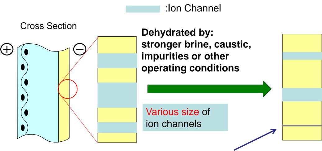
Relatively narrow channel will lose the function in strongly dehydrated state.
