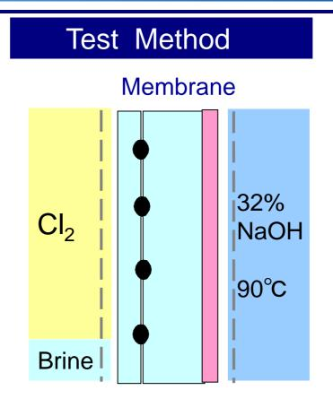
Cl<sub>2</sub> gas stagnation on anode side and high caustic strength on cathode side. In this condition, membrane will have salt crystals.
