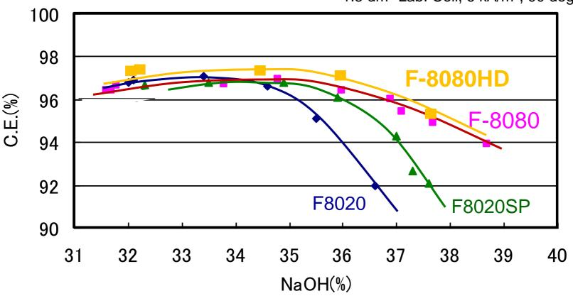
F-8080 series keep good current efficiency over widest range of NaOH strength
