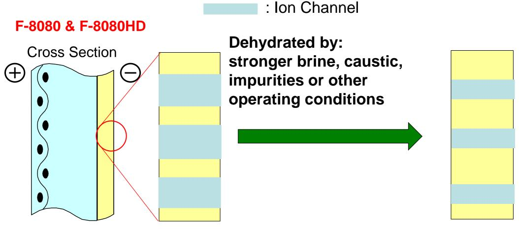
Due to uniform channel size, ion channels with uniform size do not lose function
