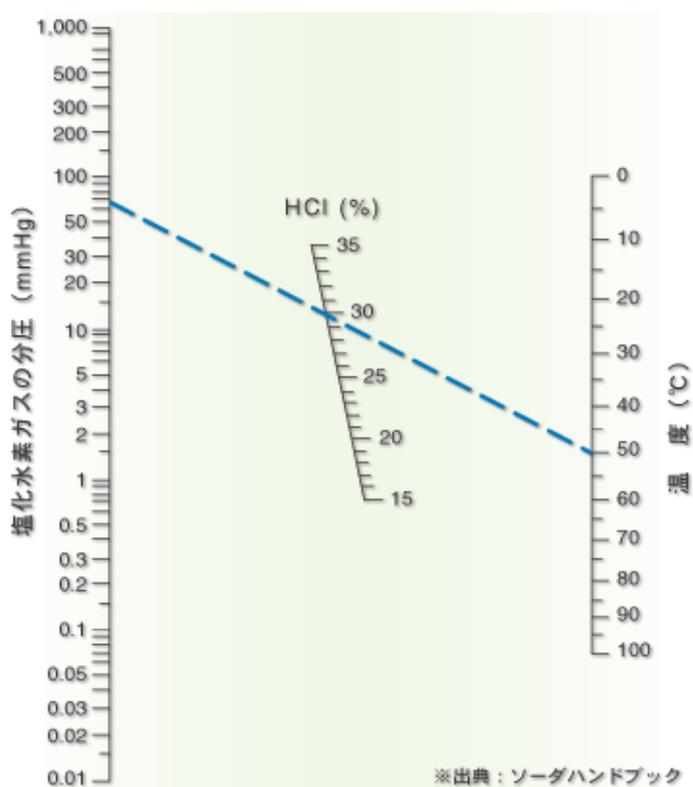
(注) NOMOGRAPH FOR PARTIAL PRESSURES OF HYDROGEN CHLORIDE
